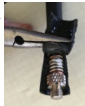
Peeling back the outer coating of the Laird antenna
