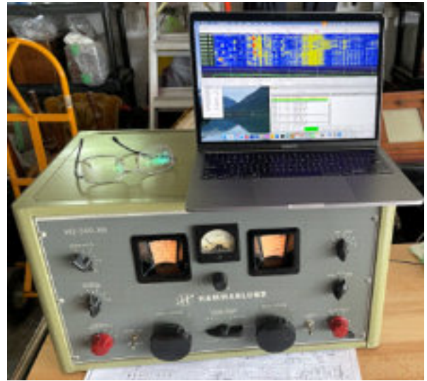
Figure 3 – Decoding FT8 Through the Receiver’s Speaker
