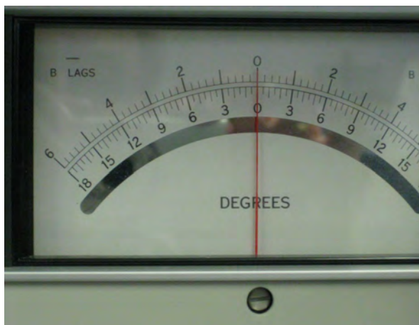
Foto 4 Schaal Fasemeting HP8405A Vector Voltmeter
