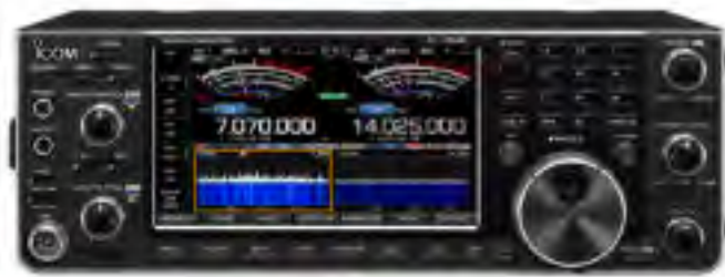
ICOM IC-7610 transceiver. On my IC-7610, the RIT controls are conveniently located in the lower right-hand corner.
