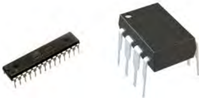
Figure 10 – AtMega328 and PIC12F629 Micro-controllers [11]
