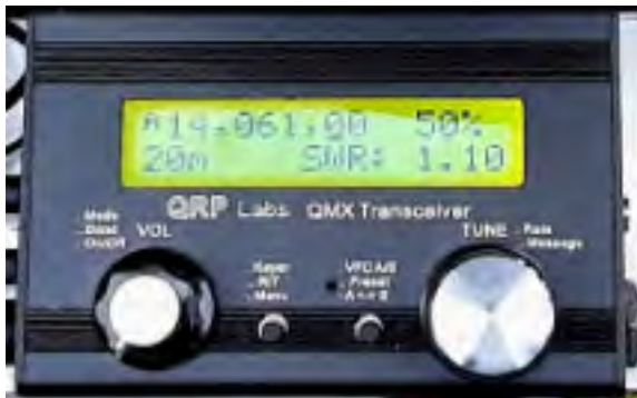
SWR on the deck 2 feet above ground
