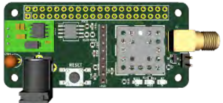
Rendering of the a prototype IP400 HAT board. Note that the metal shield on the right side next to the antenna connector is the radio.
