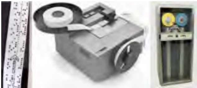
Figure 11 – Perforated Tape; Paper Tape reader; 7-Track Magnetic Tape Drive
