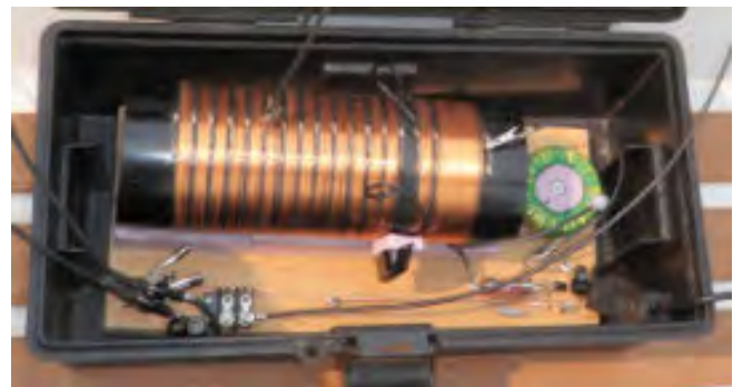
Figure 5: Variometer coil with multiple taps (left) and matching transformer (right).
