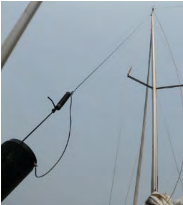
Figure 3 [above]: Base loading coil and 38' sloping vertical antenna
