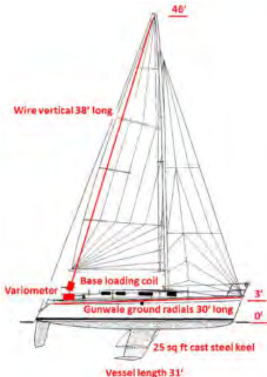
Figure 4 [below]: General arrangement of antenna and ground radials on the boat.
