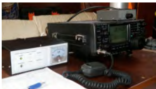
Figure 6: Set-up with VE7CNF power mixer transverter on the left and HF transceiver IF on the right.
