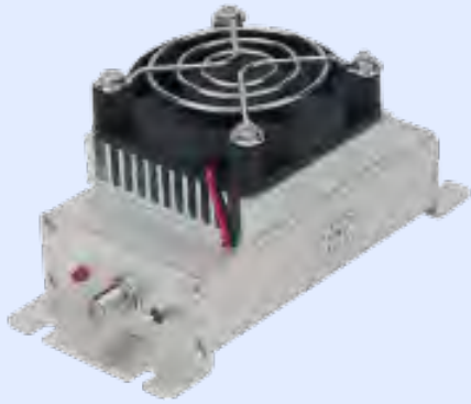
OutStar RF Power Amplifier Modules, available on eBay, typically about $60-70 ea. 70cm RF Linear Power Amplifier, P(dtv) = 0.9 W 2.5 Mhz - 1.2 Ghz
