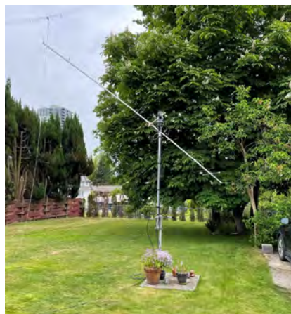
Figure 2 – Mast-mounted 12-element Yagi
