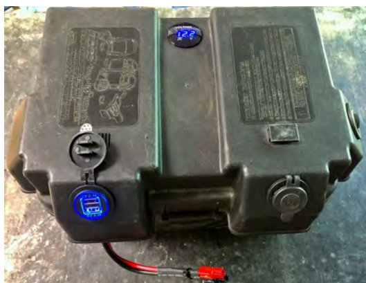
Above: The closed box with the switch, meter, USB charging ports and 12 volt accessory socket. Below: Internal wiring with the circuit breaker, one main heavy gauge wire and four Powerpole accessory sockets.
