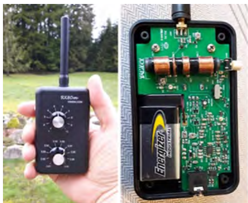
Second generation 80m receiver designed by Les VA7OM
