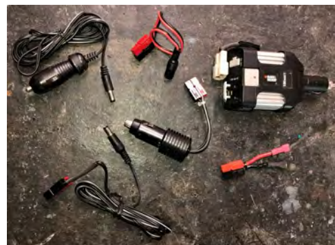
Above: There are lots of useful accessories, such as this LED 12-volt light. Below: My collection of handy jumpers and adapters for various configurations I might need. Note the small inverter to provide 110 volts at 100 Watts.
